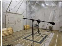
Picture 3 and 4: Loudspeaker and Microphones for  $L_{W0}$  measurements All in all 2 loudspeaker positions and 8 microphone positions for each one of these.
