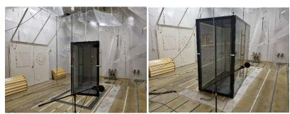
Picture 1 and 2: Test Object in the test room. 2 positions for L<sub>W1</sub> measurements All in all 2 object positions and 8 microphone positions for each one of these
