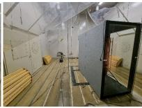
Mesurement of  $T_0$  and  $T_1$  according to ISO354.
